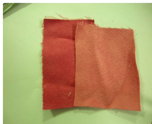
Figure 5. Different color tones of polyester microfibers, dyed at 95 °C under identical conditions with and without IL (left and right, respectively) (original unmodified photo).
