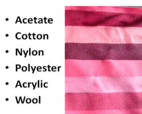
Figure 6. Multifiber fabric dyed with disperse Red 13 (0.5%) at 95 °C (atmospheric pressure) in the presence of IL (2 g/L) (original unmodified photo).
